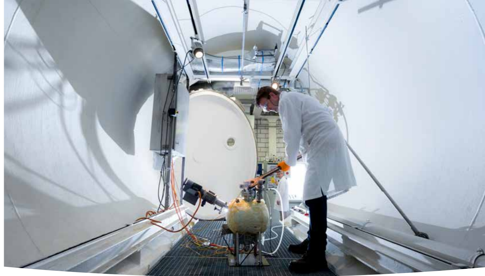
55 m 3 total containment tank for large-scale safety testing in Deventer, the Netherlands
