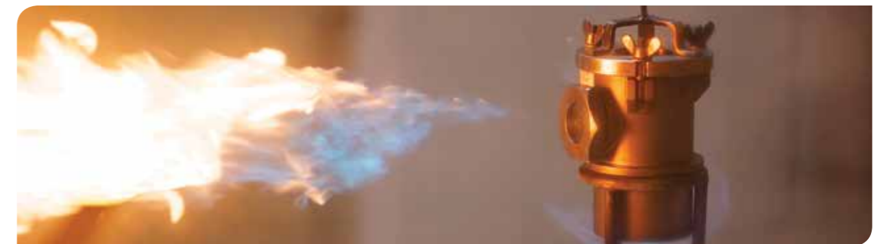
Safety testing to determine the sensitiveness of peroxides to the effect of heat under confinement
